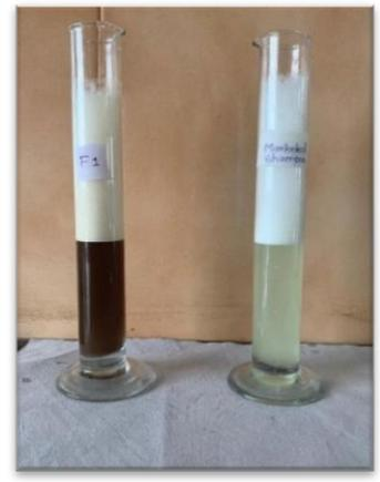
Fig. 11: Dirt dispersion test
