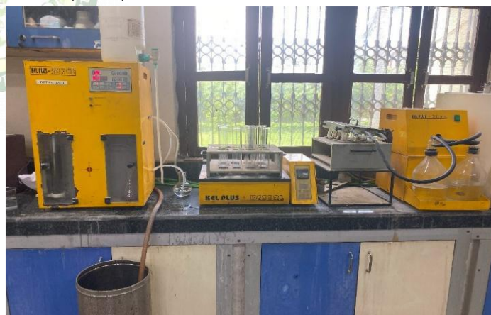
Fig.3- Protein Analysis through Kjeldahl method
