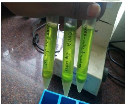
**Fig.7** 6.0gms  $MgSO_4$  anhydrous and 1.5gms sodium acetate anhydrous was added and for 10 min by hand
