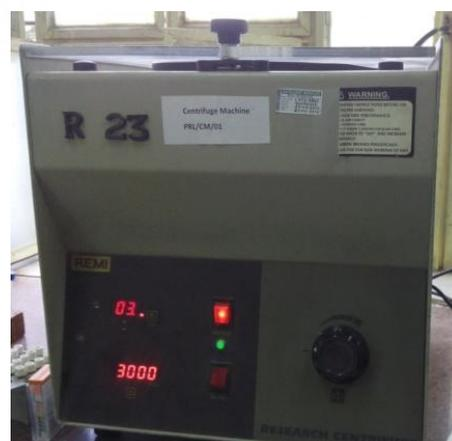
**Fig.8** After shaking the sample was centrifuged at  $> 1500$  rpm to shake vigorously separate the solid material
